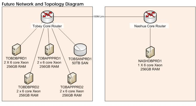
When the above configuration was designed DoIT, NHES and the current NHUIS vendor participated in the review and also performed usage and volume analyses so the system would be properly sized for all its components and some future usage growth.
